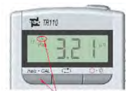
Press the Left Key for a long time, the tester will enter the status of Mean Value calibration and a symbol CAL will display on screen
