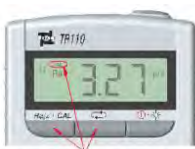
Under CAL status, press the Left Key to increase the value by turns and press the Middle Key to decrease the value
